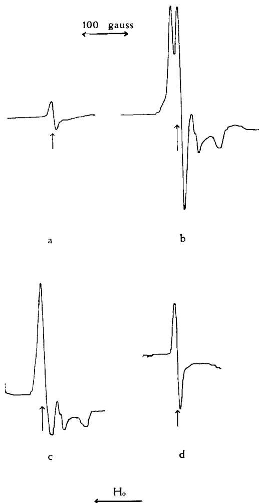
Fig. 1. Room temperature EPR spectra of wool fibers (the vertical arrow indicates g = 2.003 ): (a) naturally occurring EPR spectrum for wool fibers; (b) spectrum for wool fibers after grinding in a dry nitrogen atmosphere (sample packed in quartz tube, evacuated and sealed), this spectrum is a superposition of a \cdot\text{CH} doublet and the complex curve of -\text{CH}_2\text{S}\cdot radical; (c) sample (b) after exposure to dry oxygen for a few hours (the doublet has changed to a singlet while the -\text{CH}_2\text{S}\cdot spectrum remains unchanged); (d) same as (c) after a few days' exposure to dry oxygen (the -\text{CH}_2\text{S}\cdot spectrum has vanished, leaving only the singlet).
